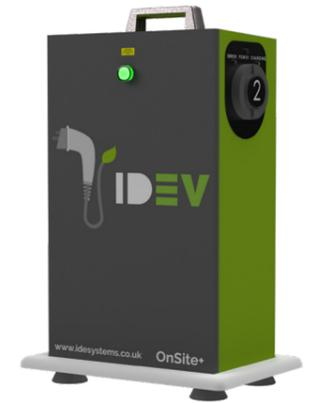
The Onsite+ has 6 mA DC residual current detection and PEN loss detection in the unit. It should be connected to a 63 A 3 Phase supply with suitable overload and 30 mA earth leakage protection.
